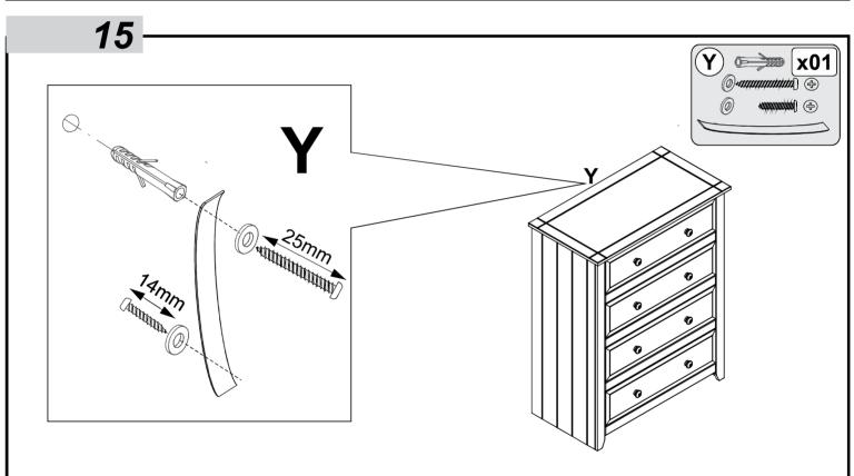
WARNING: CHECK FOR HIDDEN PIPES AND CABLES BEFORE DRILLING.
