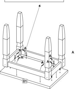
Glue must be added to the dowel holes on part 01
