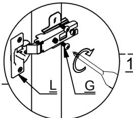
1. VERTICAL ADJUSTMENT VIA SLOT IN TH MOUNTING PLATE
