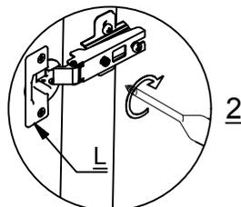
2. LATERAL ADJUSTMENT BY SCREW ADJUSTING
