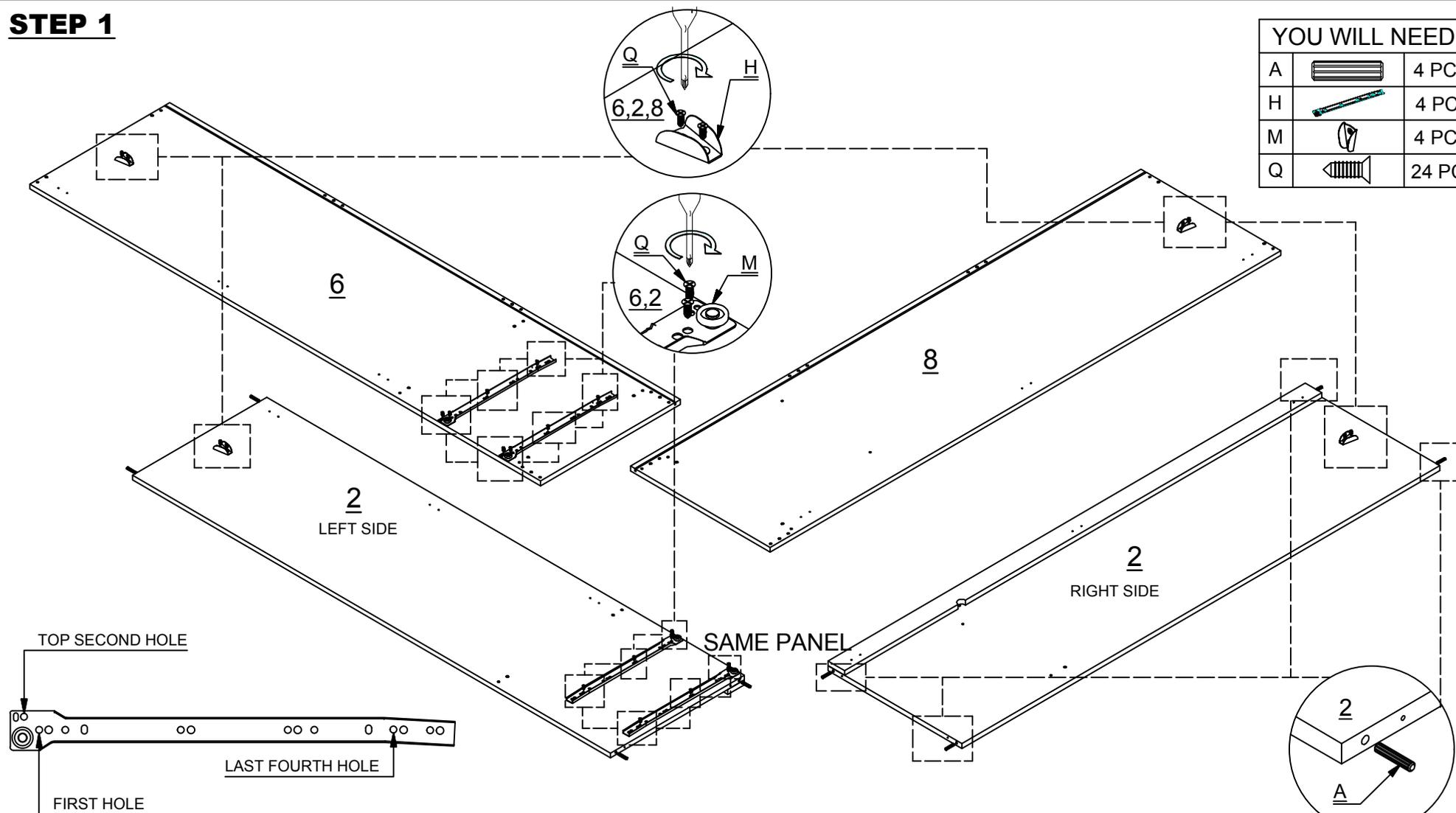
**SCREW MUST BE INSERTED IN THE FIRST HOLE ON THE DRAWER RUNNER**
