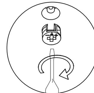
STEP 1 - PUSH CAM BOLT INTO INSERT
