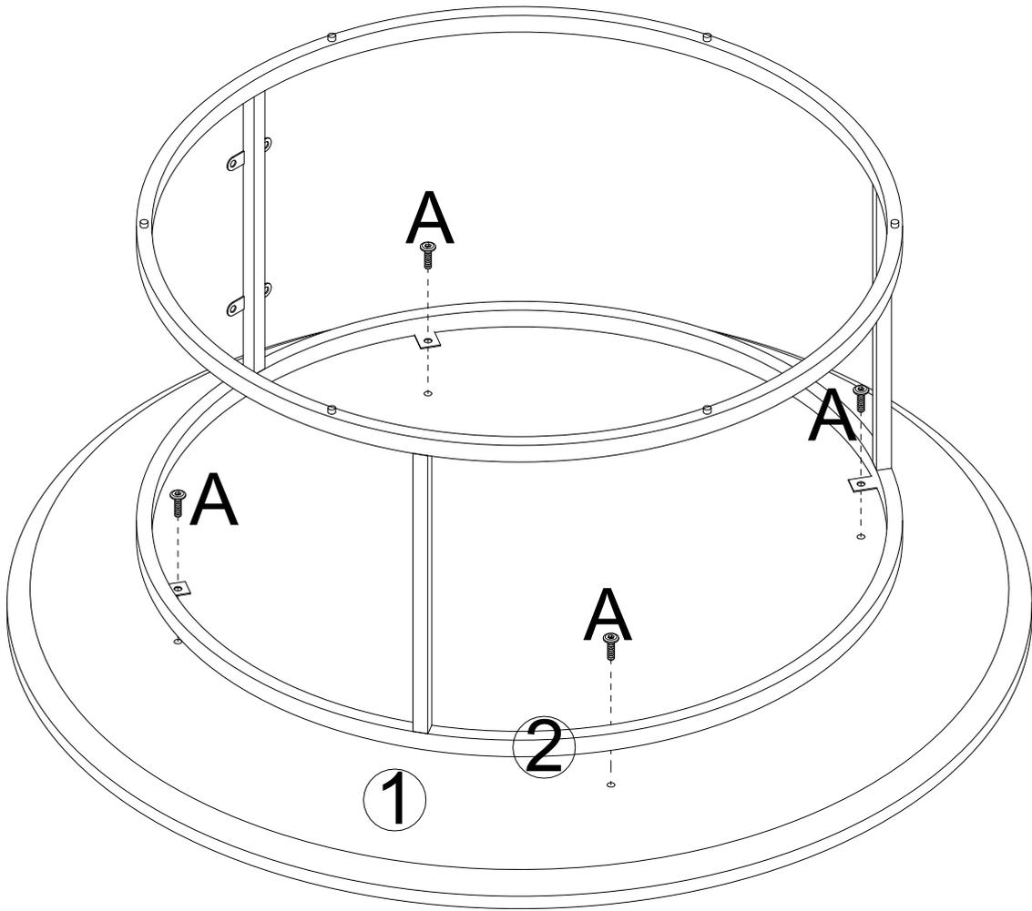
**STEP 3:** Ensure the position of the cladding plate align with the holes in the iron pipe.
