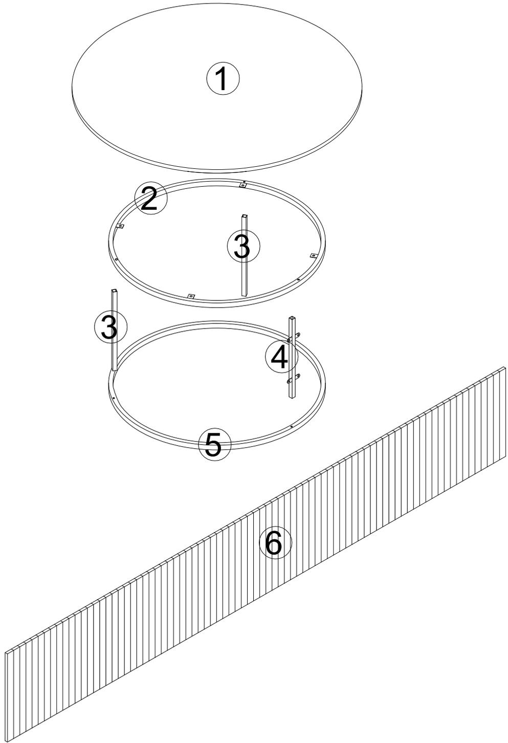
**STEP 1:** Secure 2 x metal support tube (3) and 1 x metal support tube with ear (4) with top & bottom metal frame (2),(5) by 6 x screw (D) with allen key (C).
