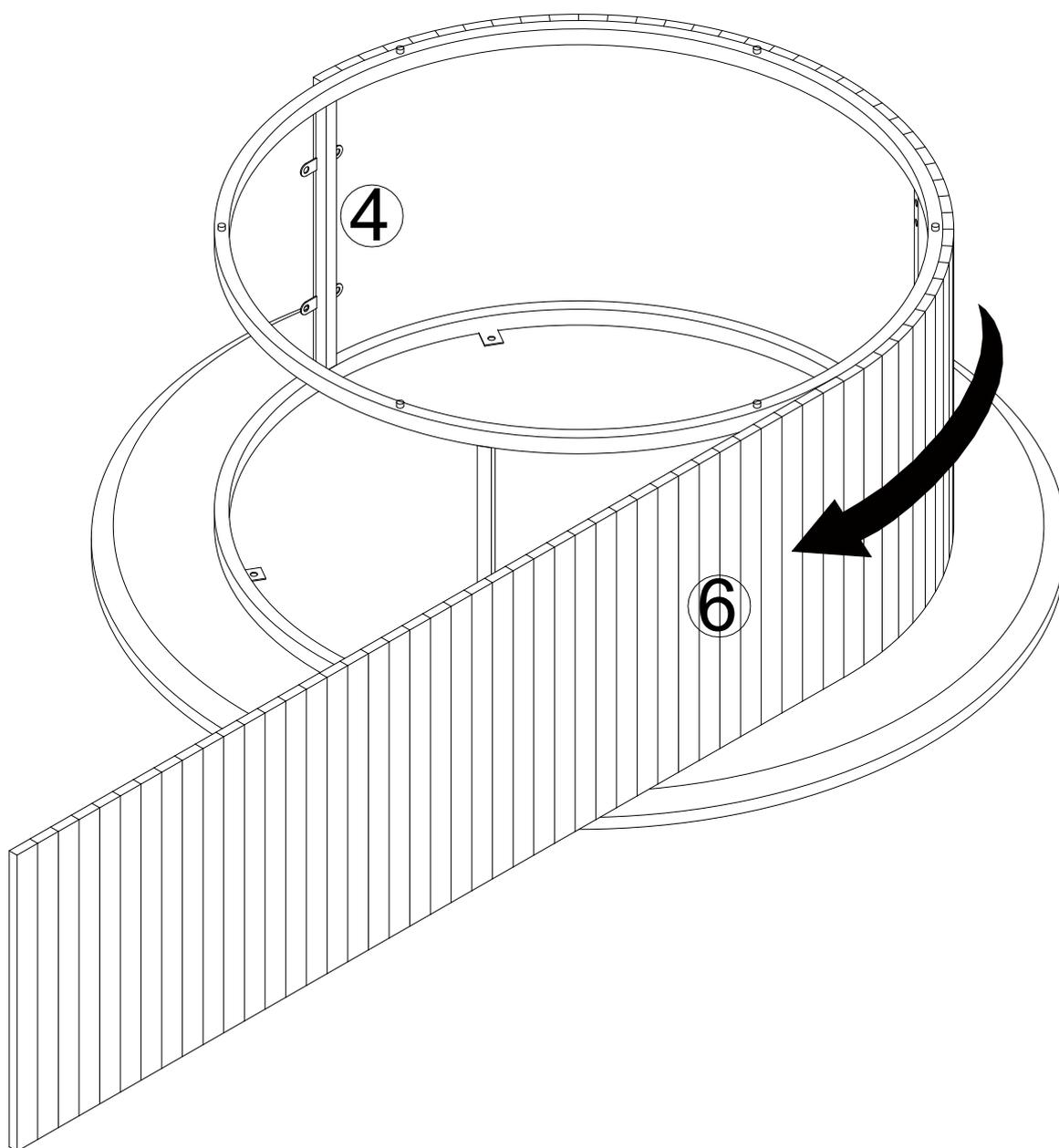
**STEP 4:** Secure the metal support tube with ear (4) with cladding plate by 4 x screw (B).
