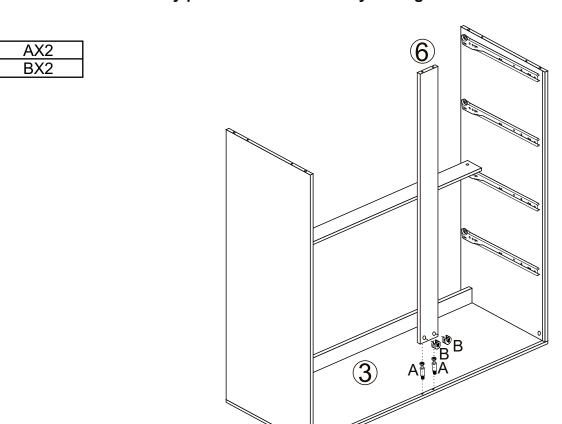
STEP 6:Attach two back panels(8) before assemble the bottom panel;
