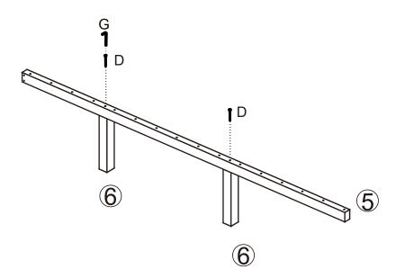
Step 4: Attach centre rail(5) in to bracket B,and screw with hardware C.
