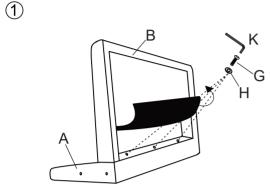
Step 1: Place the seat platform (B) on the back panel (A) and lock it with bolts (G)(H).
