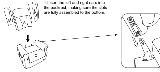
2.Gently push down until the back locks into the position. Insert the back(A) on the Base(C) over the two gliders.
