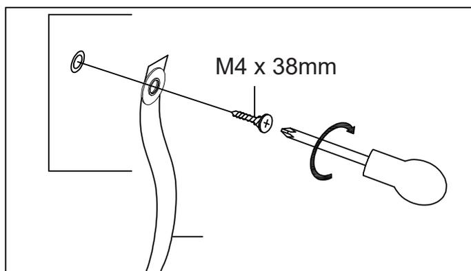
**NOTE:** Wall fixing are not supplied with this product as different wall materials require different types of fixing devices (such as Rawl plugs on bricks wall). You must use fixing devices suitable for the type of wall you intend to mount this product to. Please ensure that the head of any screw used has a diameter greater than the diameter of the mounting hole on the product and that the fixing is safe and secure before use.
