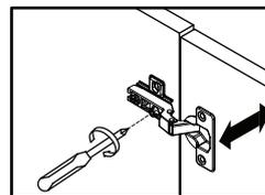
**A. Lateral adjustment by screw adjusting**
