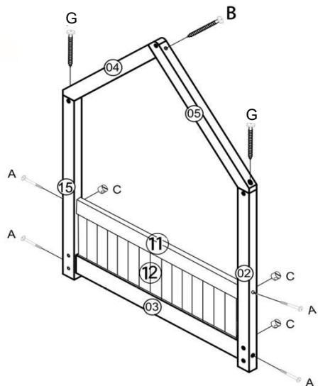
Step 3: Attach the 1 x Front right corner panels (1) and the 1 x Back right corner panels(16) to the 1 x Bottom head rail (3), 1 x Top head rail (11) and1 x Head Panel (12)using hardware parts (A) and (C). Then attach the 1 x Back right roof panel (6) and 1 x front right roof panel (7) using hardware part (B)and(G).
