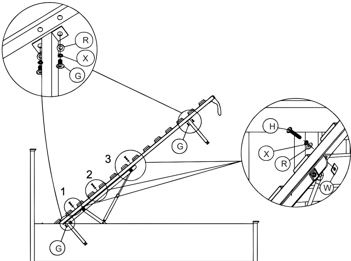
Step 8: Adjust the bed base making sure that the distance to the footboard is approximately 15mm to above . Tighten all bolts and screws now.
