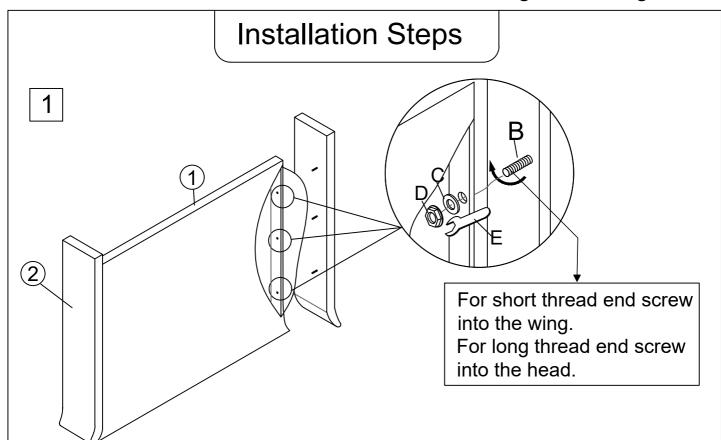
Turn the top of Headboard(1)&Wings(2) upside down on the ground.Attach the Lead screw(B) into the Wings(2) firstly. Then mount both Wings(2) to Headboard(1) by pushing the Washer(C) and Hex Nut(D) to fit . Tighten Hex Nut(D) with Solid Wrench(E).
