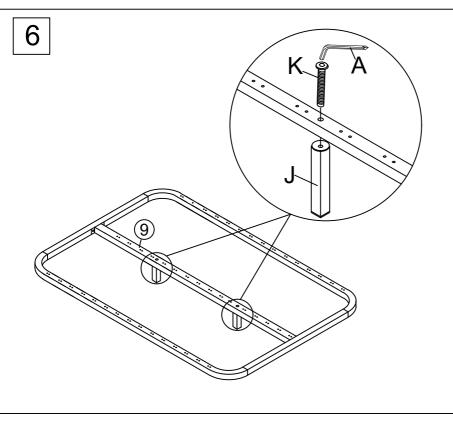
Use Allen Key(A) To fix the Central Legs(J) under the Metal Central Beam(9) with Bolts(K).
