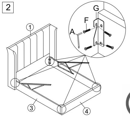
Attach the Bracket (G) with Bolt (F) and slightly tighten with Allen Key (A). Mount both Siderails (3) to Headboard (1) and Footboard (4) by pushing the Bracket (G) down to fit. Do not fully tighten the screws at this moment.
