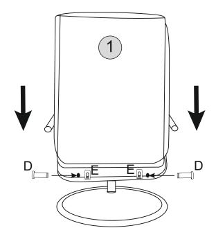
UNFOLD CHAIR UNTIL THE THREE HOLES LINE UP, NOW INSERT PUSH CLIP BOLT.
