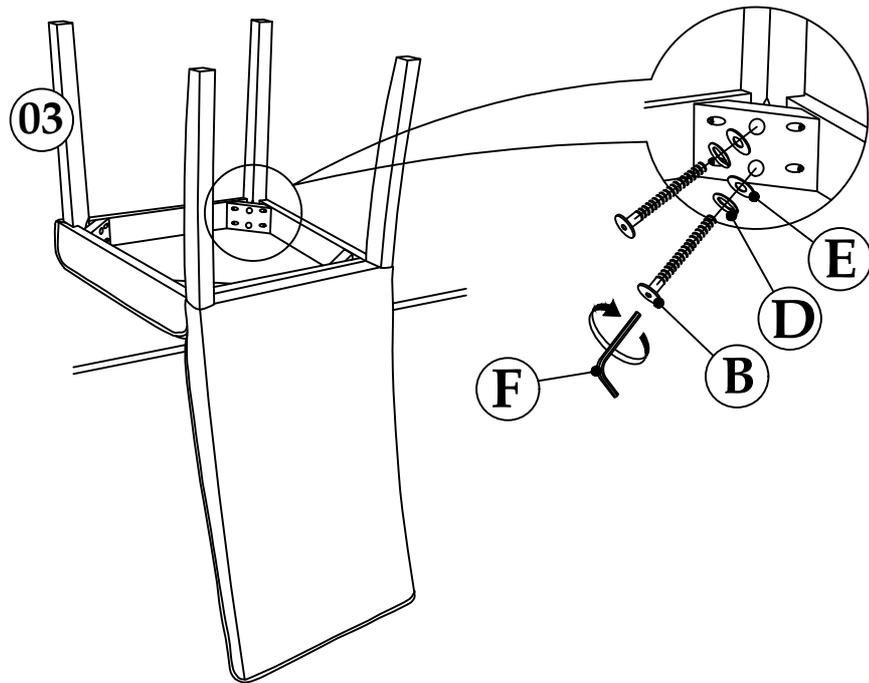
**IMPORTANT** Carefully turn the chair upright and place on a flat surface. Make adjustments to ensure that the chair frame is straight and that the legs are even on the floor then **FULLY TIGHTEN ALL BOLTS** assembled in previous steps using Allen key (F).
