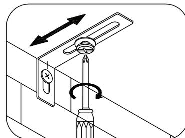
**NOTE :** Wall fixing are not supplied with this product as different wall materials require different types of fixing devices (such as Rawl plugs on brick work). You must use fixing devices suitable for the type of wall you intend to mount this product to. Please ensure that the head of any screw used has a diameter greater than the diameter of the mounting hole on the product and that the fixing is safe and secure before use.
