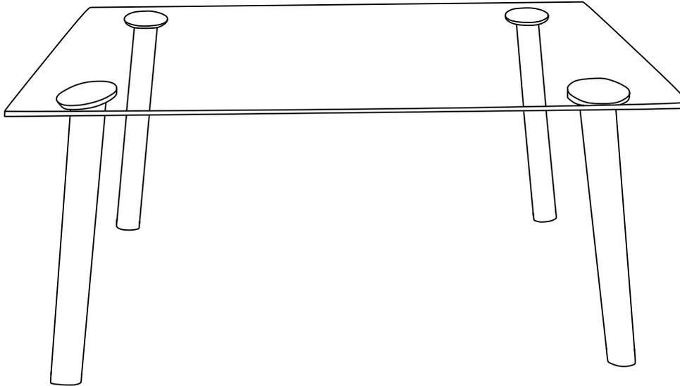
THIS PRODUCT INCLUDES TOUGHENED GLASS WITH A NOMINAL THICKNESS OF 8MM. IF THE GLASS IS CHIPPED OR BROKEN PLEASE REPLACE WITH TYPE DESCRIBED OR ALTERNATIVELY CONSULT WITH THE RETAILER STATING THE MODEL DETAILS.
