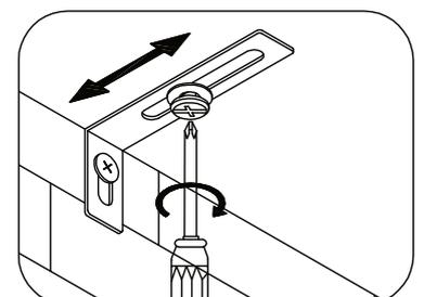
**NOTE :** Wall fixing are not supplied with this product as different wall materials require different types of fixing devices (such as Rawl plugs on brick work). You must use fixing devices suitable for the type of wall you intend to mount this product to. Please ensure that the head of any screw used has a diameter greater than the diameter of the mounting hole on the product and that the fixing is safe and secure before use.
