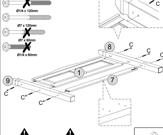
Please assemble on a clean soft surface to avoid damage. Glue must be added to the dowel holes on part 8 and 9.
