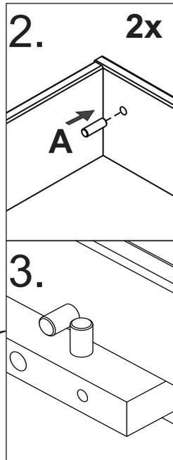
2; Push wooden dowels in through the pre-drilled holes close to the back of the drawer sides until they are level with the inside edge of the drawer sides.
