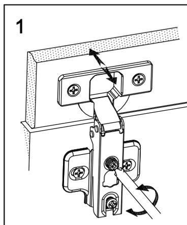
Once flaps have been adjusted, tighten screws (E) to secure hinge mounting plates in their final position.
