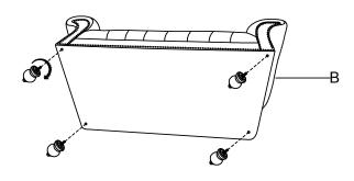
Step 2: Screw the foot (B) into the bottom of the product as shown.
