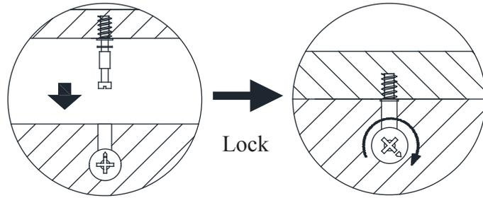
Use a flat blade screwdriver to tighten the cam nuts. A quarter turn clockwise is all that is needed.
