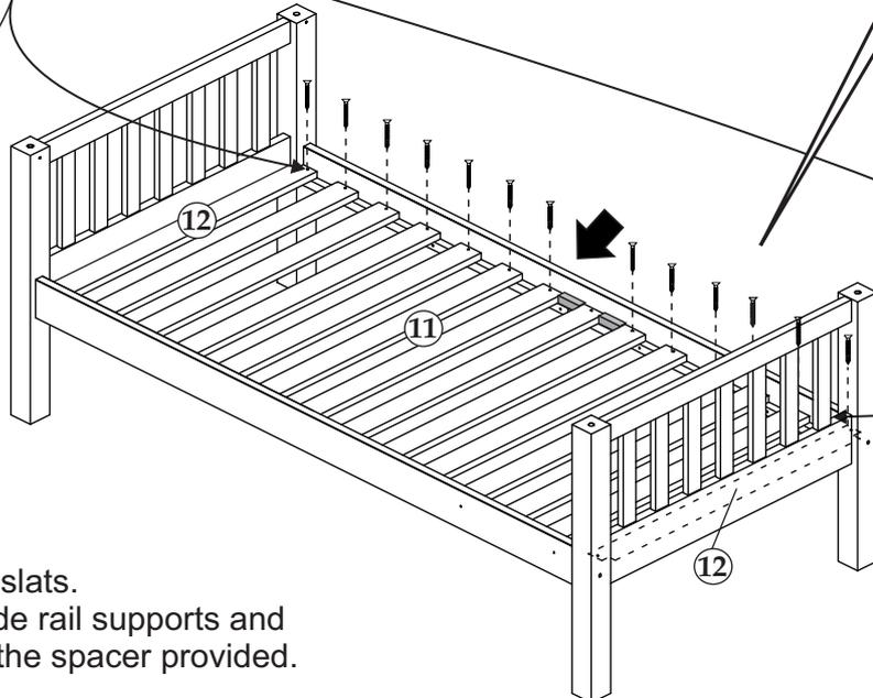
Next attach the remaining slats. Place the slats onto the side rail supports and distribute evenly by using the spacer provided.
