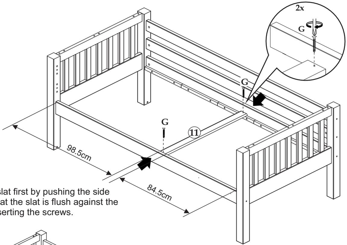
Attach the centre slat first by pushing the side rails together so that the slat is flush against the side rail, before inserting the screws.
