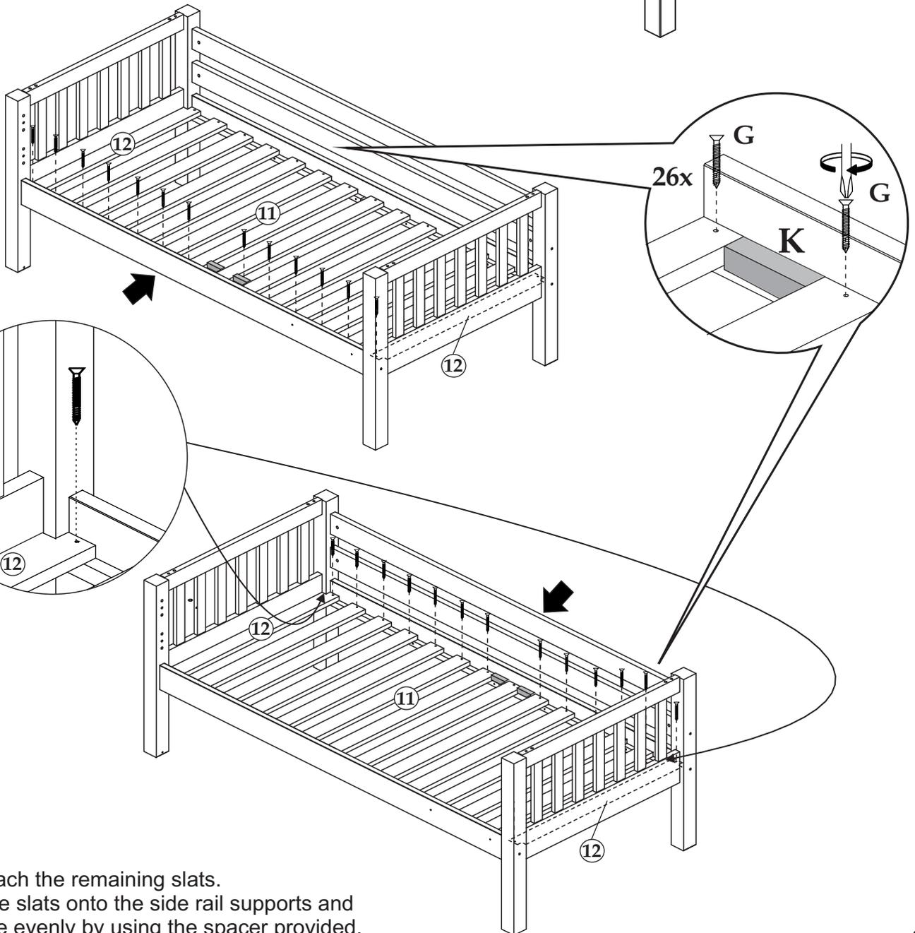
Next attach the remaining slats. Place the slats onto the side rail supports and distribute evenly by using the spacer provided.
