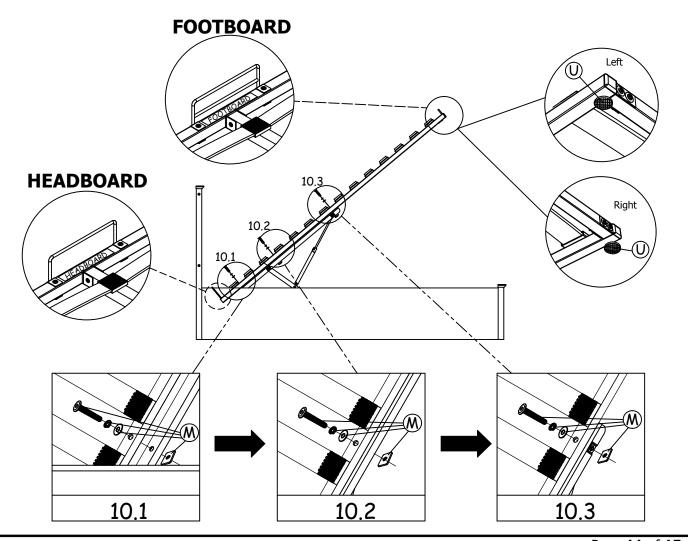
**Step 11**: Tighten all bolts and screws now. Top view of assembly bed. DO NOT use any power tools as this may damage the frame and will invalidate any claim.
