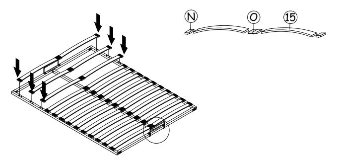
**Step 10**: Assemble the bed base on the right & left hydraulic frame and fix bolts  $\bf M$  starting from ' 10.1 ' to ' 10.3 ' as shown and stick it the self adhesive  $\bf U$  as shown.
