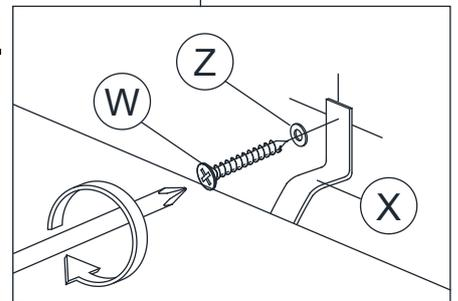
4. Add safety strap (X), washer (Z) using 3.5 x 16mm screw (V) to back of cabinet.
