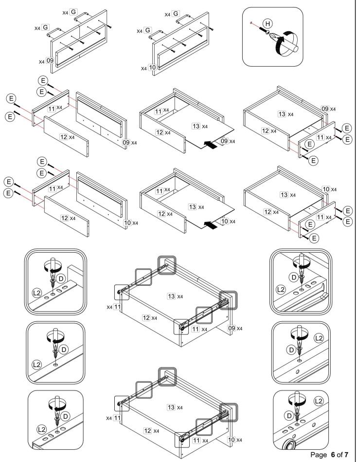
Step 10: Assemble the drawers in place along the drawer slides.
