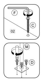
Step 7: Attach hardware K1 into panel (1), (2), (3) and (4) using hardware K2 with a screwdriver (not provided).
