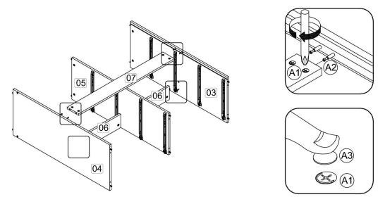
**Step 4:** Attach the panel (3), (4) and (5) to panel (1) using hardware A1 and A3 with a screwdriver (not provided). **DO NOT** use any power tools as this may damage the frame and will invalidate any claim.
