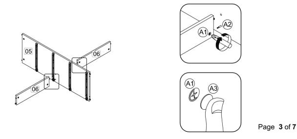
Step 3: Attach the panel (6) and (7) to panel (3) and (4) using hardware A1 and A3 with a screwdriver (not provided).
