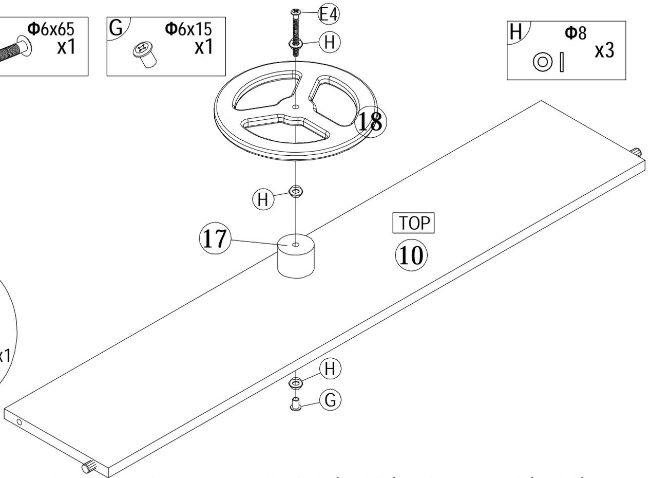
Using 2 cross head screwdrivers, ensure the bolt (part E4) and captive nut (part G) are tightly and securely fixed together and that the wheel can still turn freely.
